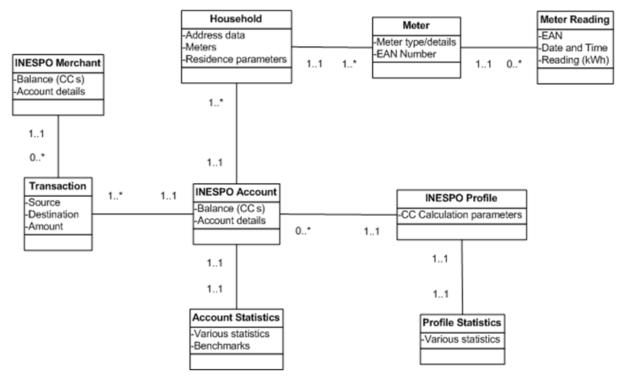
Figure 13 Back-office database class diagram
