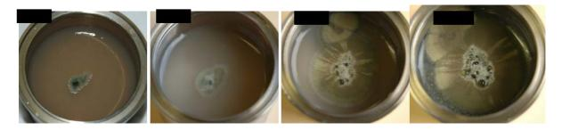
Figure 9 : Development of Cladosporium microorganisms (strain 01) over time
