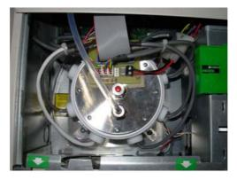
Figure 43 : E-nose sensor chamber
