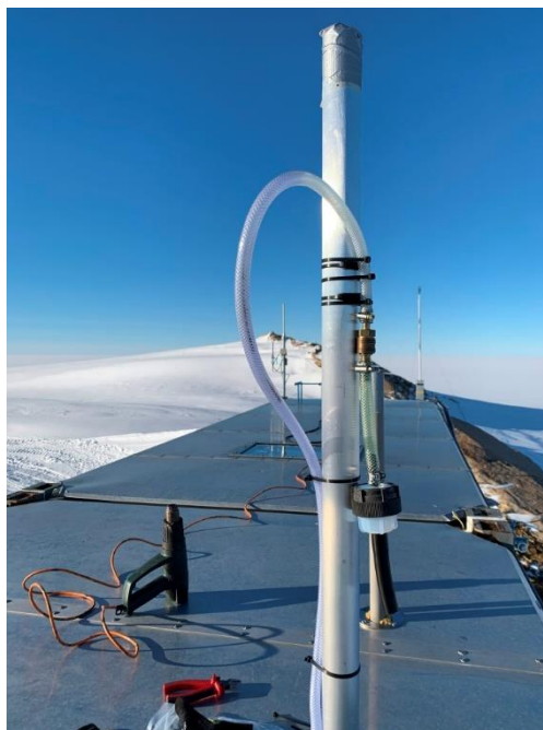
Figure 4: inlet setup for the INP sampling on the roof of the northern 'Atmos' shelter
