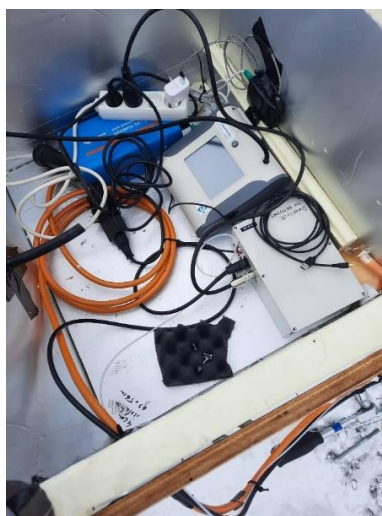
Figure 3: inside view of the box at the CLIMB remote site with OPS and other controlling devices
