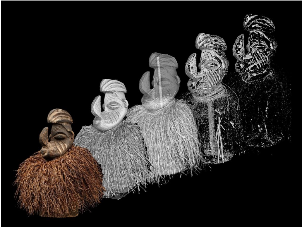
Figure 4: From left to right a Yaka mask (EO.), its 3D rendering. The middle rendering is shown at 50 % transparency. The last two renderings increasingly filter out the less attenuating materials, isolating only the pigment and rope used in the mask. Rendering made using VGStudio MAX®. ©RMCA ©UGCT ©UGent-Woodlab
