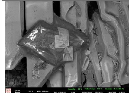
Figure 3. Example, (E)SEM image of a recrystallized salt mixture (Photo KIK-IRPA)
