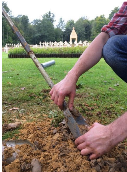
Figure 3-3 - Drilling of shallow boreholes was accomplished through the utilization of a hand auger.
