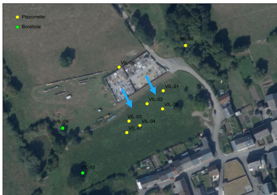
Figure 4-4. Placement of the piezometers (yellow dots) at the Villers-Deux-Eglises site, along with a general indication of the groundwater flow direction (blue arrows). The additional boreholes (green dots) were carried out to gather localized data for the geological model.
