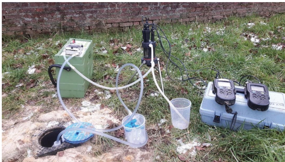
Figure 3-4 –Extracting water samples from a piezometer and in situ measurement of field parameters using a flow cell and field electrodes.
