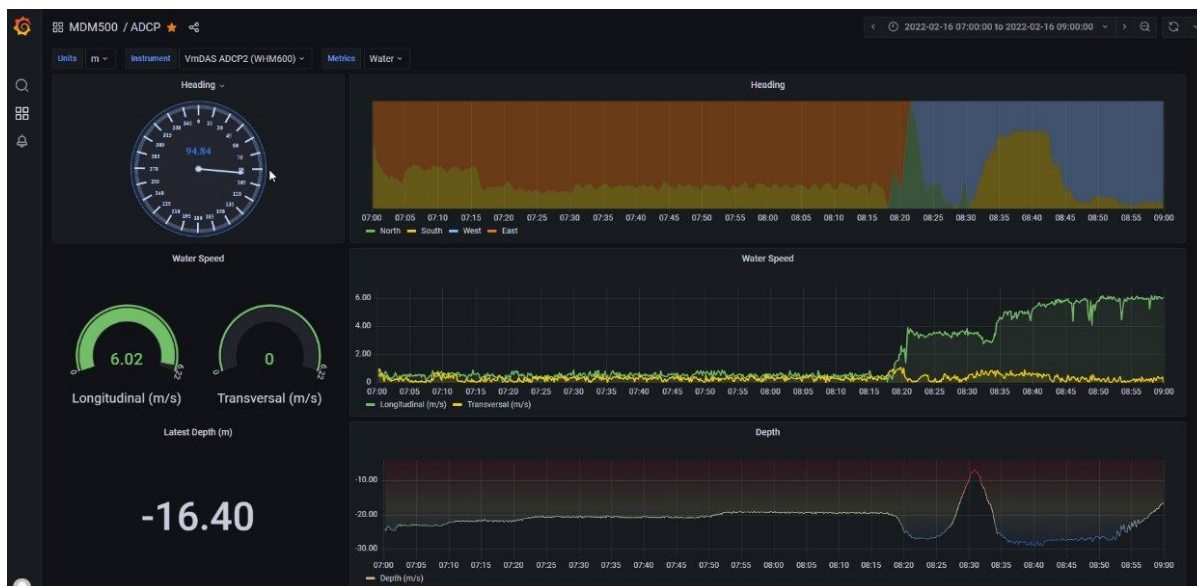
Figure 5: Example of the Grafana dashboard deployed on-board the RV Belgica for a real-time data visualization. This represents the depth measured by the ADCP sensor along with some navigational parameters.
