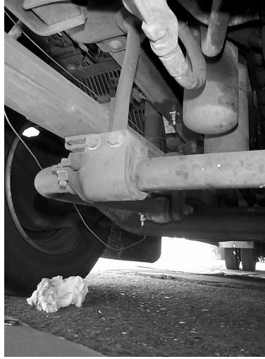
Figure 4.6: The accelerometers on the front part of the vehicle body and the front axle.
