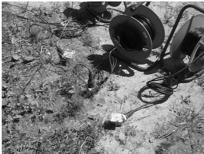
Figure 4.9: The accelerometers FF2y, FF2z and FF2x (from left to right) mounted on aluminium stakes with a cruciform cross section.
