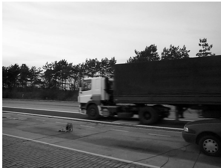
Figure 4.1: The passage of a DAF FT85 truck and trailer on the artificial unevenness at the DAF test circuit in Sint-Oedenrode (The Netherlands).
