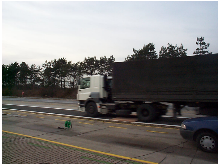
Figure 4: The passage of a DAF FT85 truck and trailer on the artificial unevenness at the DAF test circuit in Sint-Oedenrode (The Netherlands).
